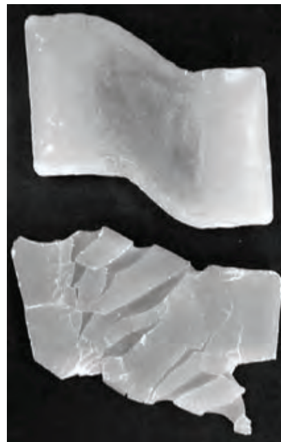
Figure 5: Blocks of wax subjected to transtensional shear. Upper is warmed block. Lower is same but ice place on surface to produce a brittle layer. The model produces features such as triangular basins, block rotations, and the possibility of traversing a path across the zone of shear that doesn't intersect any 'faults'.
