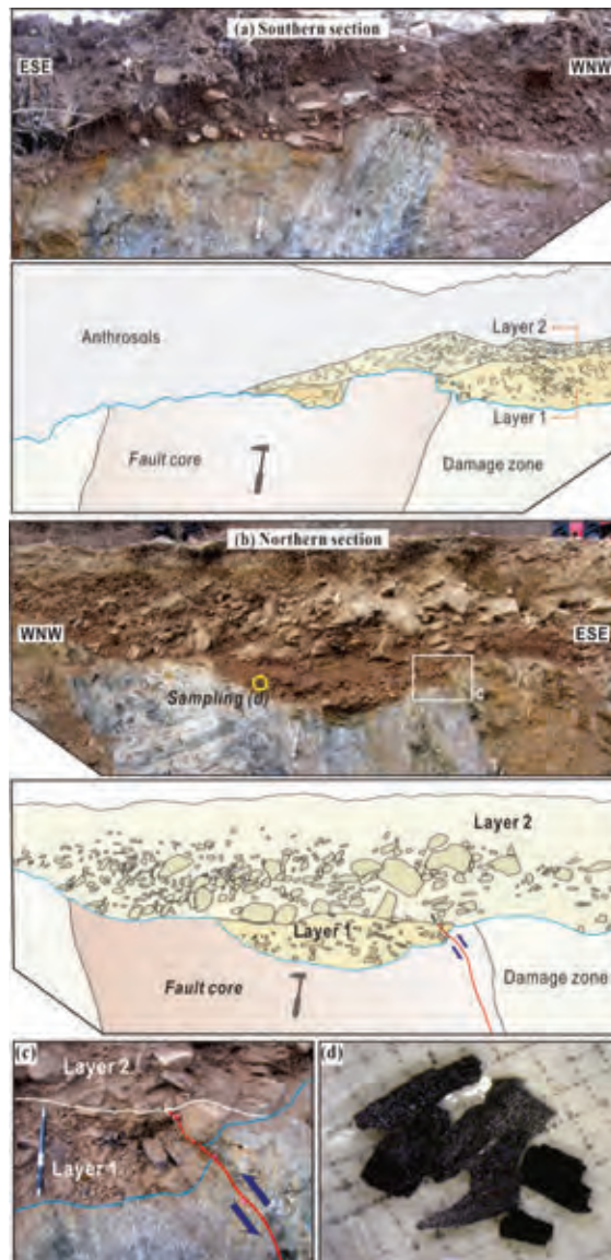
Figure 5: (a, b) Photos and sketches of the both trench walls. (c) A detailed view of the fault contact showing reverse separation. (d) Charcoals for radiocarbon dating analysis sampled in the lower layer-1, and the result indicates AD 165 ( \pm 30 ).
