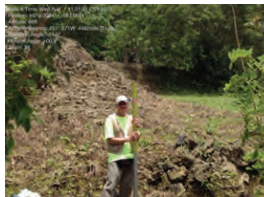
Figure 6: Example shot of the theodolite surveying of the relative vertical separation between the coral platforms.
