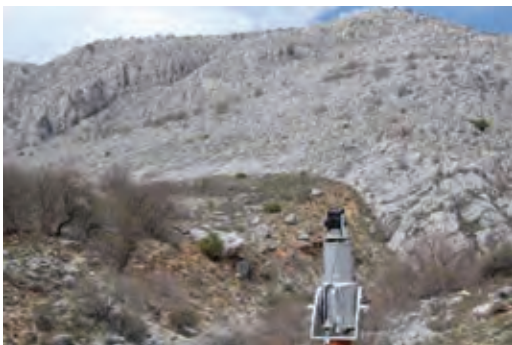
Figure 1: Terrestrial Laser scanning of the Velino-Magnola Fault, Abruzzo using a Riegl LMS420i.
