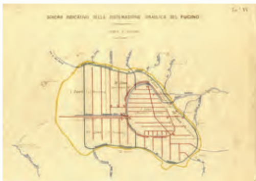
Figure 1: Hydraulic drain system for the Fucino land reclamation (Lotti et al., 1915-1916).
