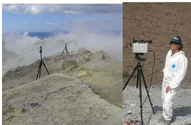
**Figure 13.** Retroreflectors (left) and tunable laser (right) on La Fossa cone.
