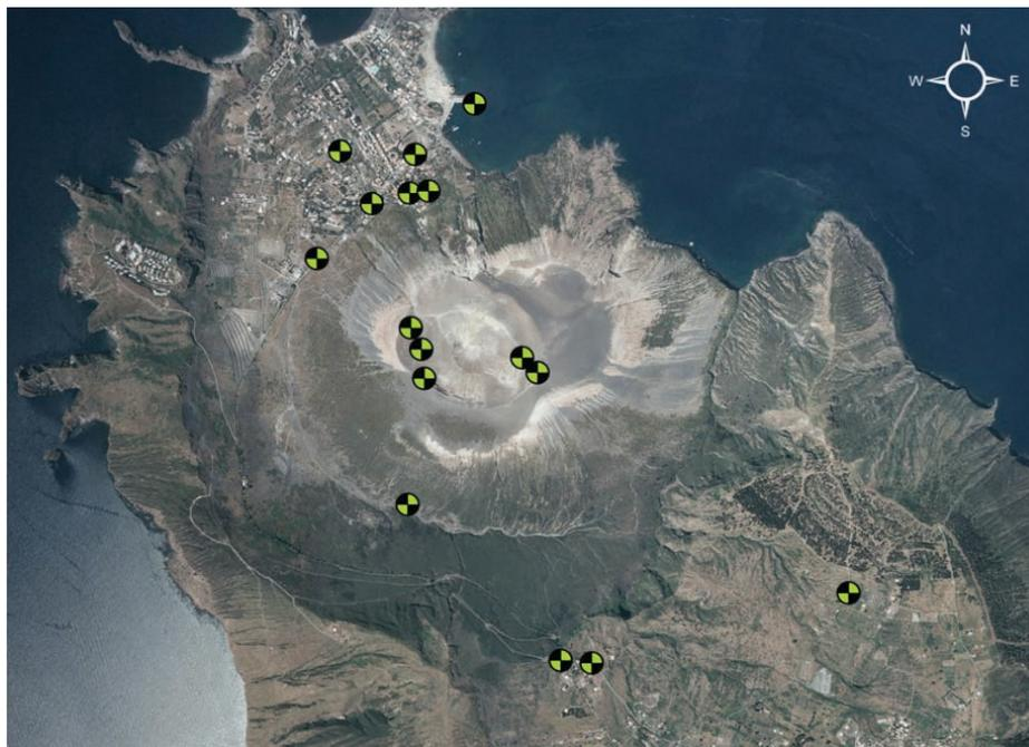
**Figure 1.** GCPs collected with GPS survey.
