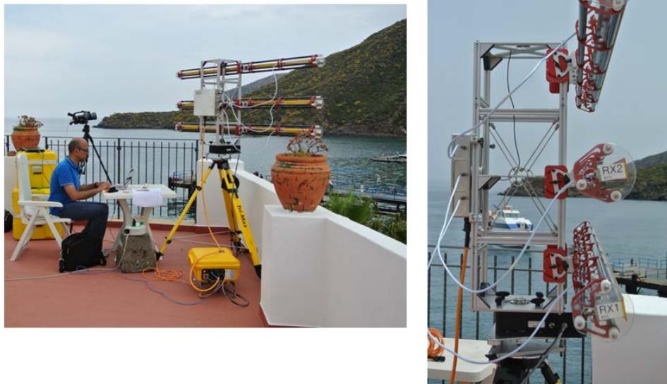
**Figure 26.** Installation GPRI-II near the thermal camera (terrace of hotel Faraglioni): details of the headframe of the GPRI-II and the equipment (three antennas, one of which transmitter and two receivers).
