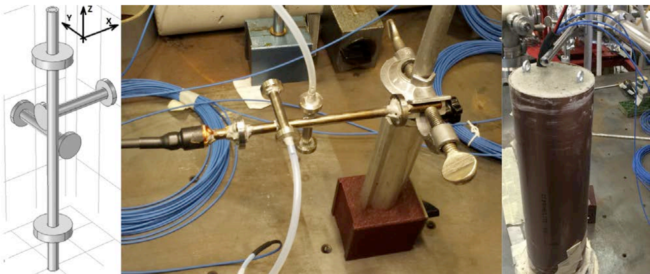
Figure 1. The multi-axial strain sensor. Left: mechanical design; centre: multi-axis prototype; right: borehole system.
