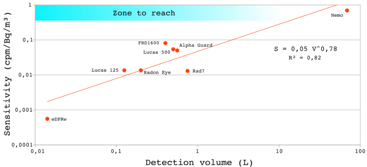
Figure 1 Sensitivity versus volume of common 222 Rn measurement devices. The zone to reach defines the specifications that an instrument dedicated to measure 222 Rn in a volcanic plume has to reach: small (< 10L for a volume device) and sensitive enough to measure low level of 222 Rn (10 Bq/m 3 ) with accurate precision (<5%) in a short time (<1h).
