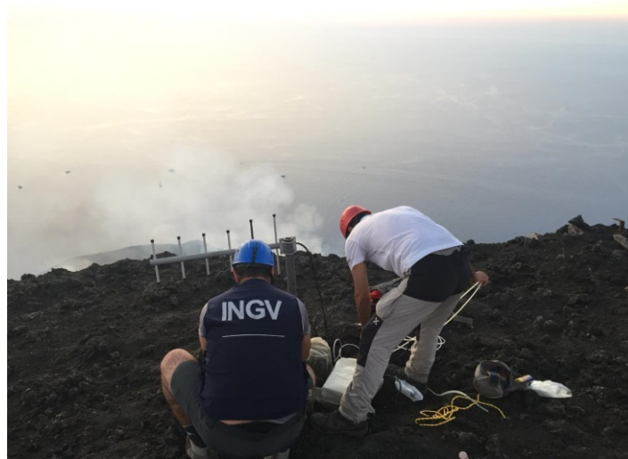
Figure 2 The C/S geochemical station installed on 20 th July after paroxysm.
