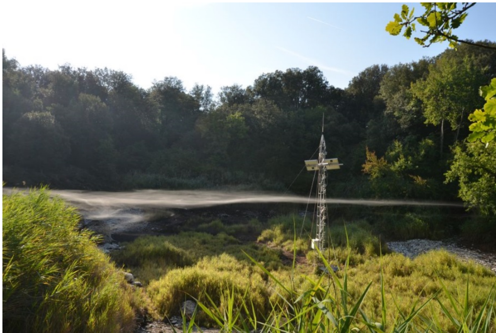
Figure 4 Inside the Bossoleto with the observation tower. The photo was done late summer morning before the desintegration of the homogeneous gas lake (75 % CO 2 ) at the bottom, below a haze that marks the upper extend of the gas lake. The autor was positioned slightly above the haze.
