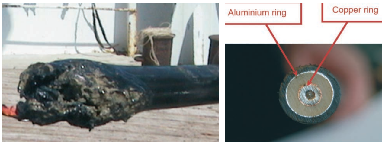
Figure 1. The cable “melted” in the epicentral area of the September 2002 earthquake (sea-floor depth 1500m): a) the cable as it was recovered; b) the cable as it had to be (after Favali et al., 2006).
