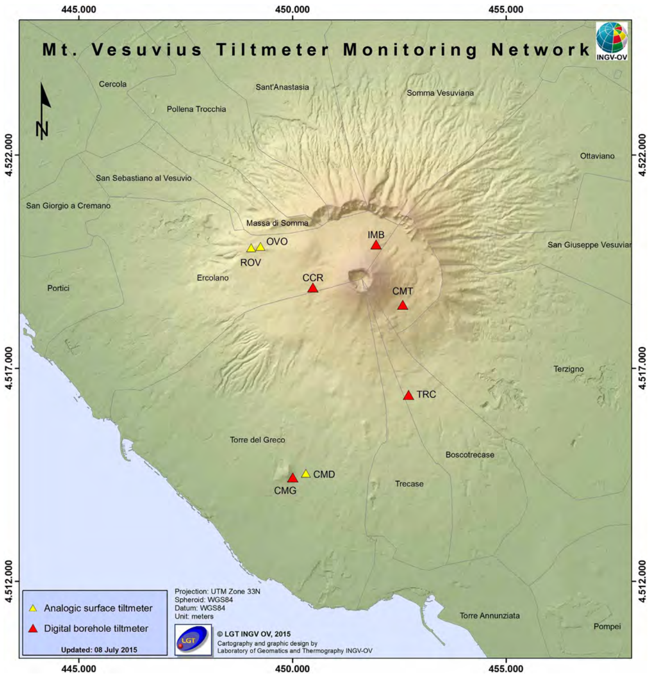
Figura 28 Vesuvio Tiltmeter Monitoring Network.
